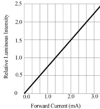
FORWARD CURRENT VS. LUMINOUS INTENSITY
